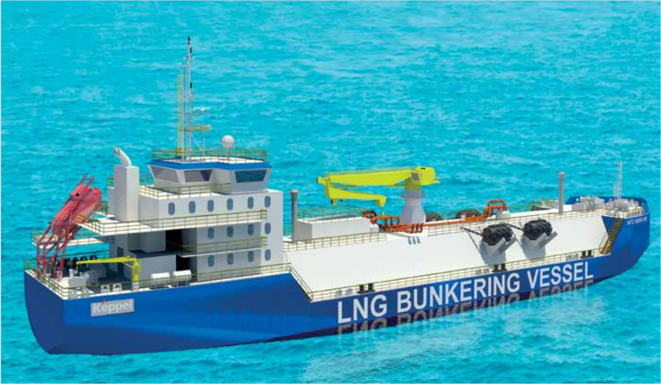
To be built to a proprietary design of Keppel O&M's ship design and development arm, Marine Technology Development, the ice-class LNG bunker vessel will have an Ice Class Arc 4 notation and a cargo capacity of 5800 cubic metres
